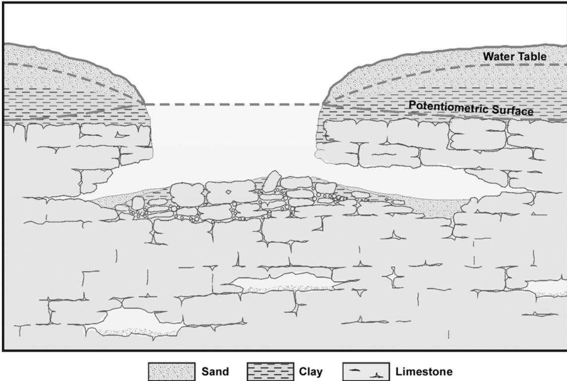
**Figure 3. Rock-Collapse Sinkhole**
