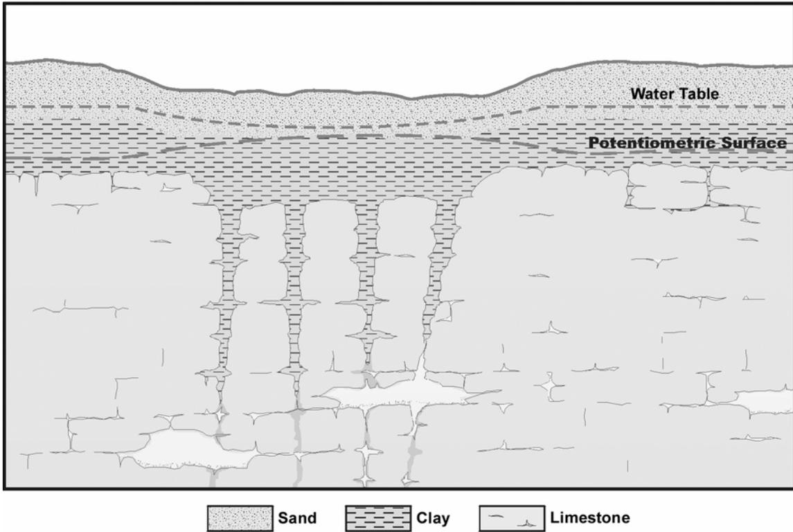
**Figure 2. Cover-Subsidence Sinkhole**
